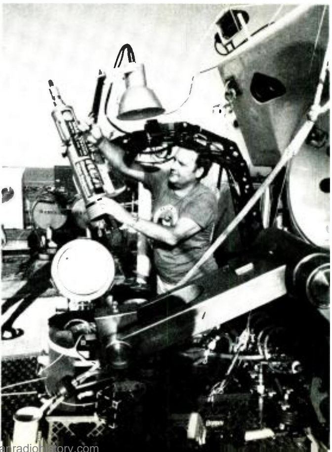
RCA technician Fred Engle makes final adjustments to mount holding the CCD camera on the mechanical arm of Alvin, before the Woods Hole research submarine is launched from its mother ship, Lulu, to probe the Galapagos Rift at the bottom of the eastern Pacific
